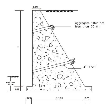
MASONRY RETAINING WALL - TYPICAL SEC.
